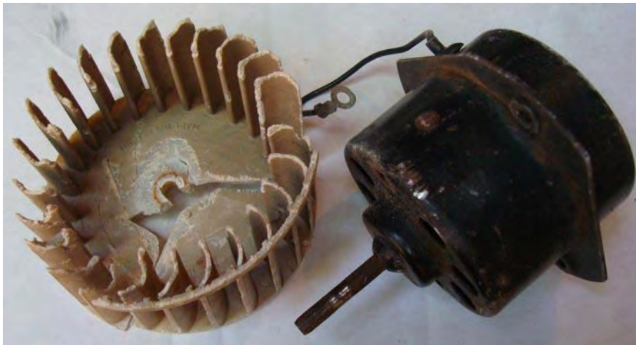
Figure 6. Photo showing the disintegrated plastic fan squirrel cage and rusty original motor.
