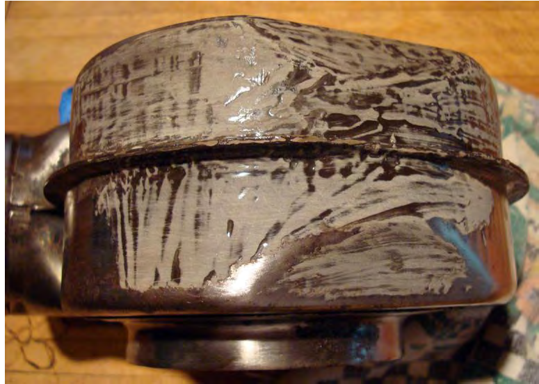
Figure 5. Photo showing base of the snail box with the sanded J-B Weld fill before priming and painting.
