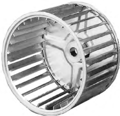
Figure 8. Indiana Fan and Fabrication replacement squirrel cage Part No. 02895776: 4.25" diameter, 2" height, 0.25" bore, and CCW rotation. Price: $16.87 on 13 June 2010.
