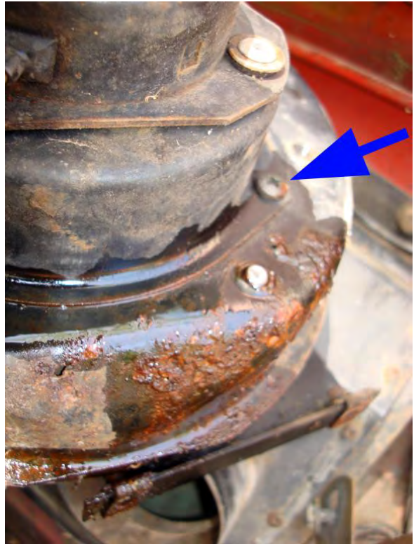
Figure 3. Base of snail box shows the extensive rust at the bottom of the box due to moisture accumulation. Three Phillips screws (one shown at blue arrow) must be removed in order to remove the cowling that the heater fan motor and squirrel cage assembly are attached to in order to replace the fan and squirrel cage and gain full access to the interior of the snail box.
