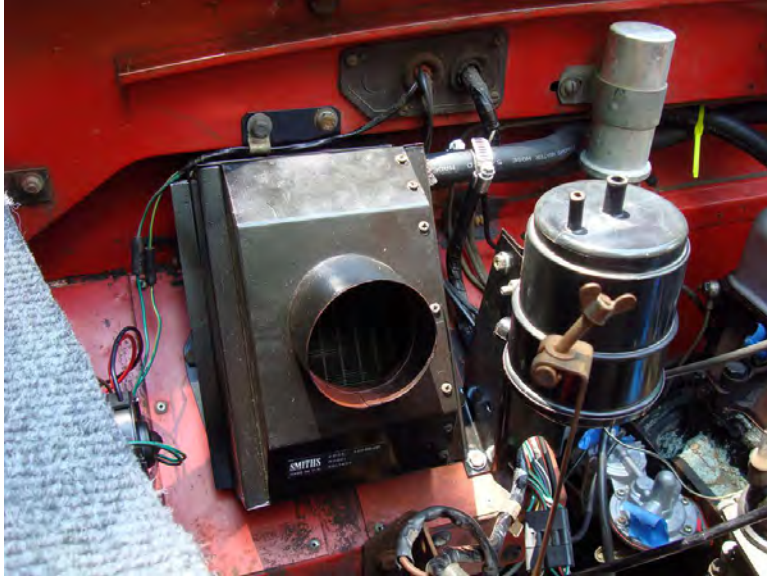
Figure 9. Photo showing heater core box reinstalled and heater hoses attached.
