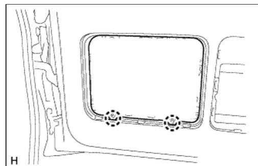
**7. REMOVE BACK DOOR INSIDE HANDLE BEZEL (for Face to Face Seat Type)**
