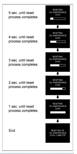
OIL MAINTENANCE INFORMATION MODE RESET OPERATION (for 1KD-FTV, for Analog Meter)
