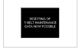
g. After the ODO/TRIP switch is turned on, enter the setting mode and change to T-BELT display mode.
