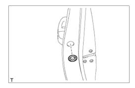
b. Using a T30 "TORX" socket wrench, loosen the screw and remove the front door outside handle cover with lock cylinder assembly.
