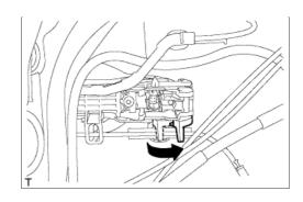
c. Remove the front door outside handle assembly as shown in the illustration.
