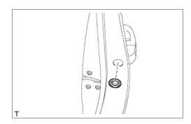
b. Using a T30 "TORX" socket wrench, loosen the screw and remove the front door outside handle cover.
