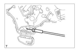
33. REMOVE FRONT DOOR OUTSIDE HANDLE FRAME SUB-ASSEMBLY LH
