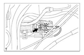
**b.** Move the lever in the direction indicated by the arrow in the illustration.
