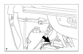
g. Disconnect the front door lock remote control cable assembly and front door inside locking cable assembly.
