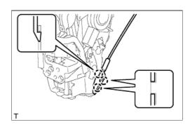
**b.** Remove the front door inside locking cable assembly.
