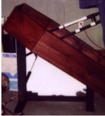
Here's a (somewhat) closer view of the mechanism. I'm using a heavy-duty screen door closer as the air cylinder. All the moving parts (with the exception of the air cylinder) are made of PVC plumbing pipe. I used about 15 feet of 3/4" pipe, a handful of tees, caps, and couplings. The body is made of 1/2" PVC and various fittings (see below).
