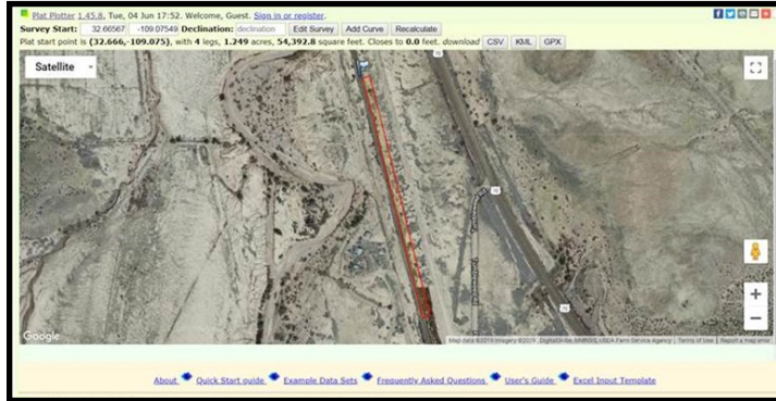
Above: Old U.S. 70 alignment, plotted using the PlatPlotter web application and the legal description provided in the Recorder's Deeds to Real Estate Book 3, page 163. Below: The same plot exported to a .kml file for display on Google Earth.
