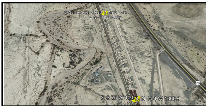
Above: Old U.S. 70 alignment, plotted using the PlatPlotter web application and the legal description provided in the Recorder's Deeds to Real Estate Book 3, page 163. Below: The same plot exported to a .kml file for display on Google Earth.
