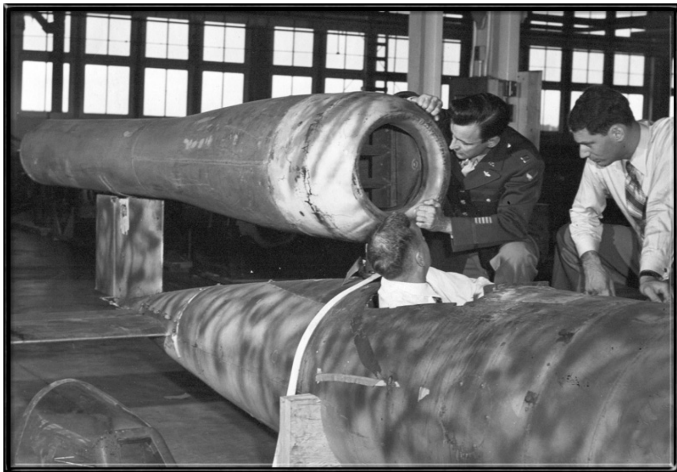
T-2 intelligence experts examine a German Reichenberg IV manned surface-to-surface missile. The Germans planned "Kamikaze" missions with these, but never carried them out.
