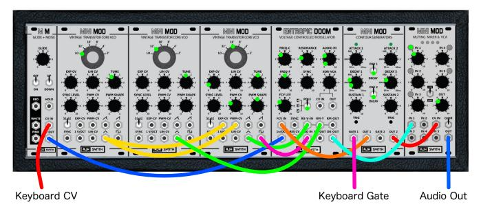
Green dots show approximate pot and switch positions. Where a pot has two dots, this illustrates the range I move them during the video. Pots and switches that do not have green dots are not used in this patch, and should be left at their zero or off positions.
