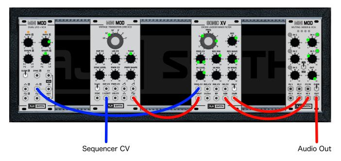
Green dots show approximate pot and switch positions. Those with two dots show the range I adjust them during the video. Pots and switches that do not have green dots are not used in this patch, and should be left at their zero or off positions.
