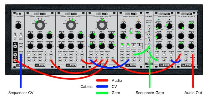
Green dots show approximate pot and switch positions. Pots and switches that do not have green dots are not used in this patch, and should be left at their zero or off positions.
