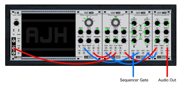
Green dots show approximate pot and switch positions, and where there are 2 dots on the same pot, this indicates the range I adjust them during the video. Pots and switches that do not have green dots are not used in this patch, and should be left at their zero or off positions.
