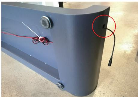
Have the cable go through L shape and the hole .
