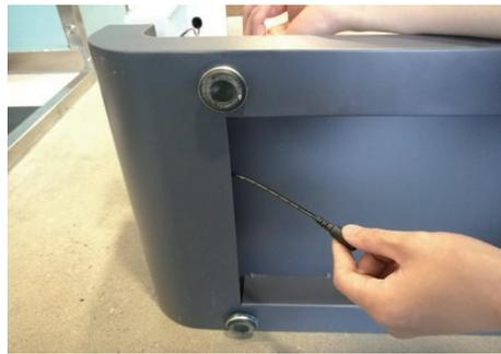
Fasten the cable at the bottom.
