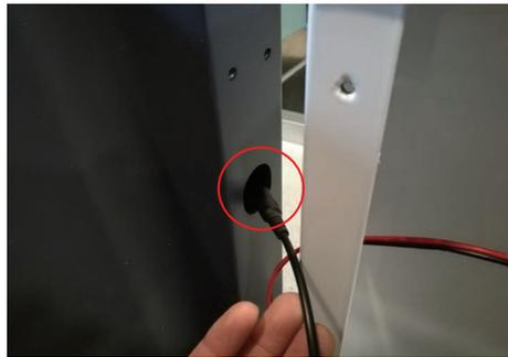
Have the cable go through the hole to get to bottom .
