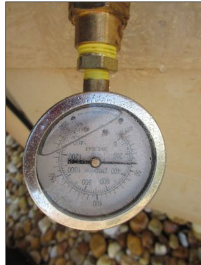
Normal water pressure at 45 PSI
