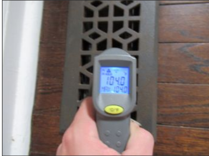
Normal heat temps at first floor
